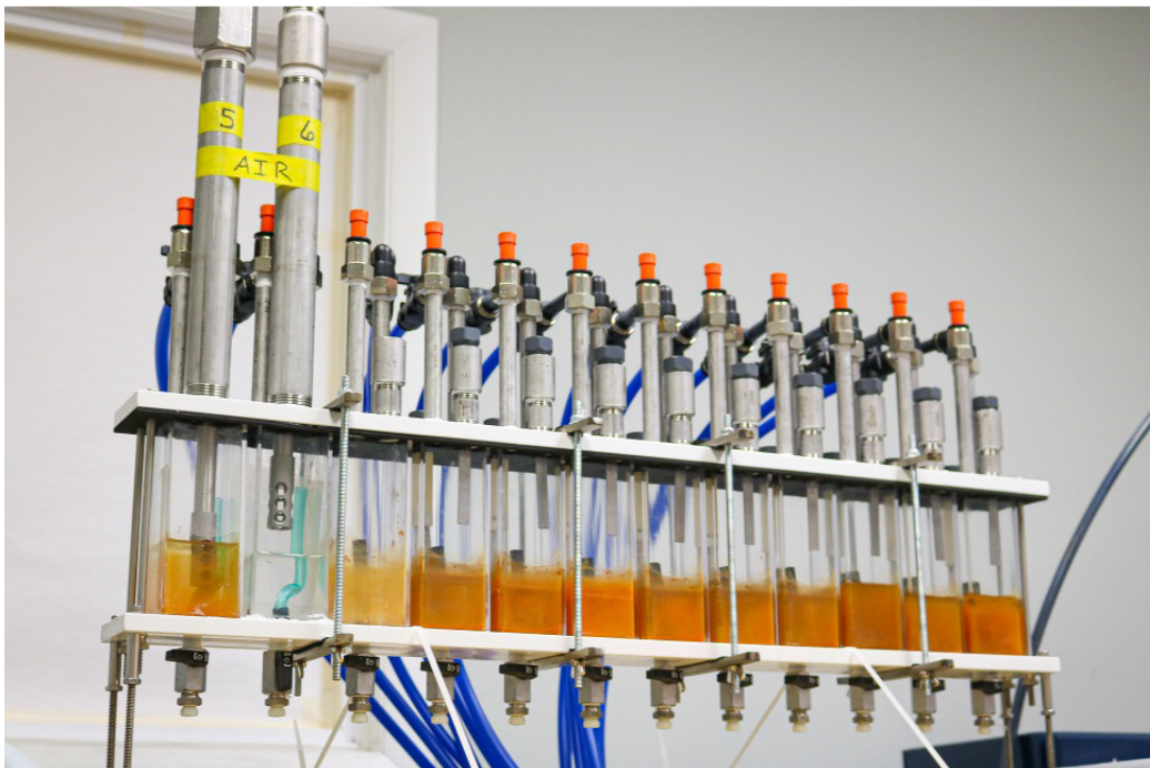
12 chambers partially filled with water where coupons made from C1018 carbon steel are submerged.
